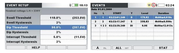
Figure 5.11: Voltage dip related screens on the instrument
