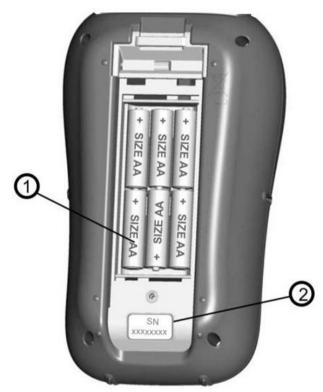
Figure 7.1: Battery compartment
