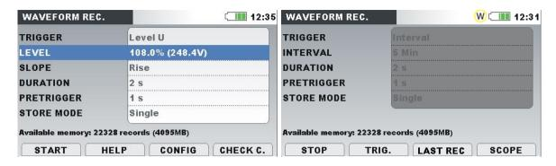
Figure 3.48: Waveform recorder setup screen
